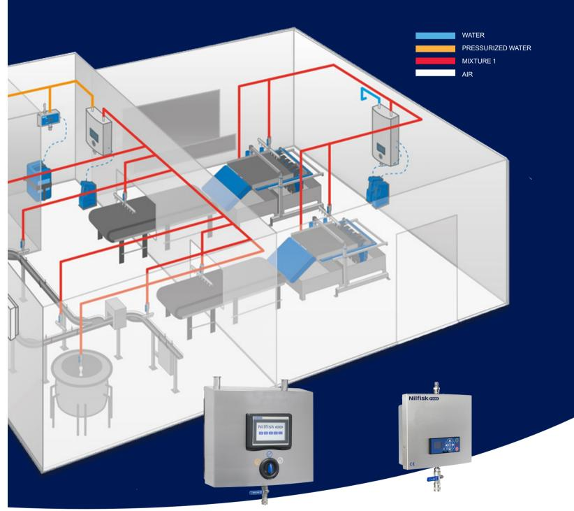
Maximum reduction of downtime used for cleaning and top of the line hygienic results with fully automated mainstations and satellites
