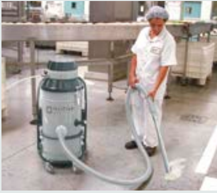
Recovery of flour in ATEX environment.
